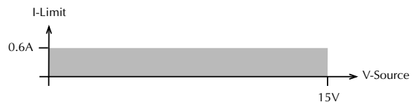
C) 500mA Measurement Range (Model 2303-PJ)
